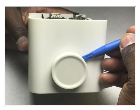
Remove the volume knob from the side of the Chumby One with a plastic opening tool.
