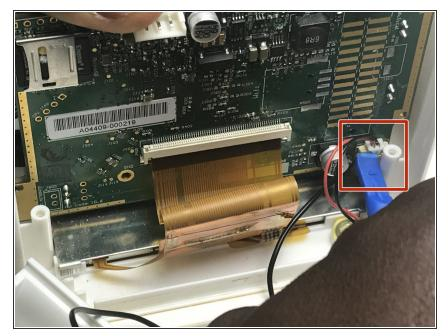
Disconnect the microphone connector from the motherboard with a plastic opening tool.
