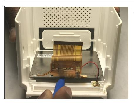
Remove the LCD screen from the outer case using a plastic opening tool.
