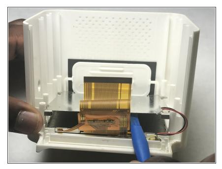
Remove the metal shield from the front case using a plastic opening tool.
