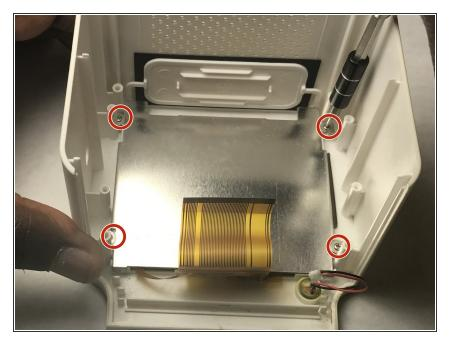
Remove the four 5.5mm screws with a Phillips PH000 screwdriver bit.
