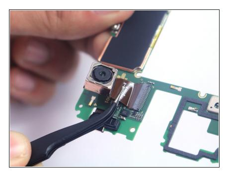
Using tweezers, pull up and remove the rear camera.
