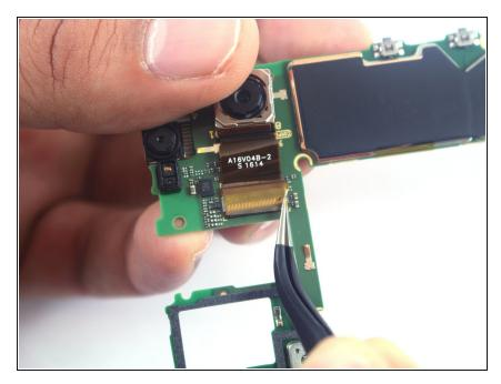
Using tweezers, remove the yellow film connecting the motherboard to the rear camera.
