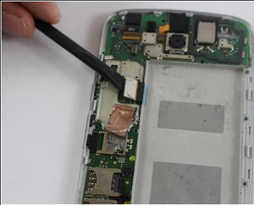
• Using a spudger, remove the two metal pieces connecting the motherboard to the front casing.
