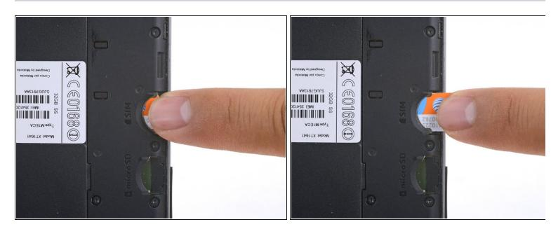
Slide out and remove the SIM card.
