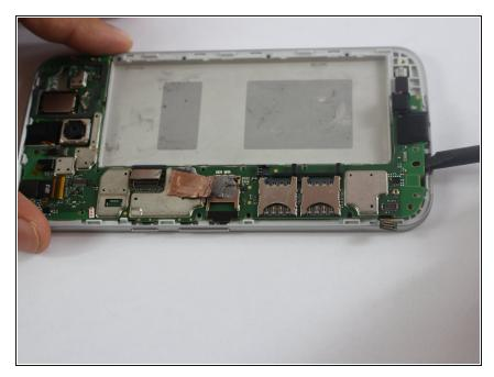
• Using a spudger, lift up and remove the motherboard.
