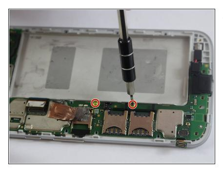
Remove two 4.0 mm T3 Torx screws connecting the motherboard to the front casing.
