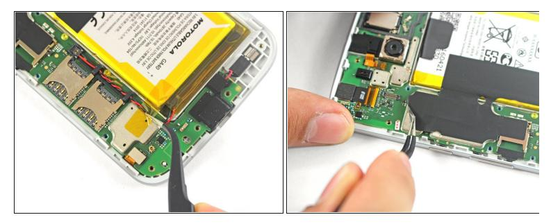
Be very careful not to puncture the battery with any sharp tools. A damaged lithium-ion battery can catch fire and/or explode.
