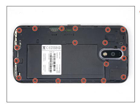
• Remove the nineteen 3.1 mm T3 screws securing the midframe.
