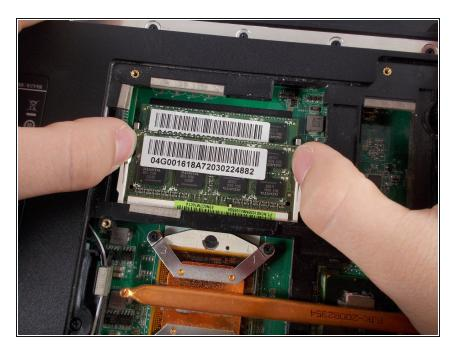
Gently push the metal retaining arms away from the center of the RAM module.
