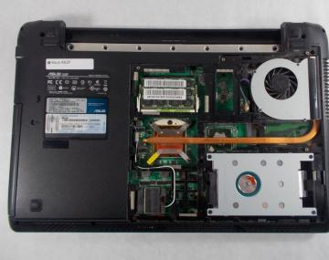
Slide the back panel away and remove the panel.
