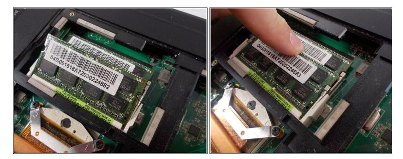
• To insert new RAM line up notch in the connector and slide in at a 30° angle.
