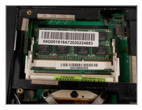
Repeat removal process for the RAM underneath.
