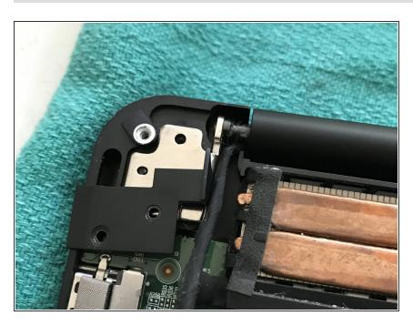
Unscrew Phillips head screws holding screen hinge.
