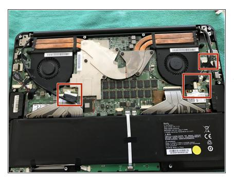
Unplug before mentioned connectors. The webcam and charger cable may require a small pry tool. The LCD cable should disconnect with a light pull on the plastic tab. The antenna cables just pop off with some upward pressure.
