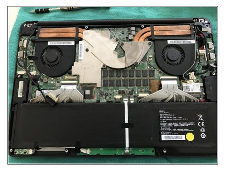
Lower case onto replacement screen, Making sure no cables get pinched in the hinge.
