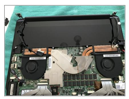
After removing screws, work the screen assembly free from the case.
