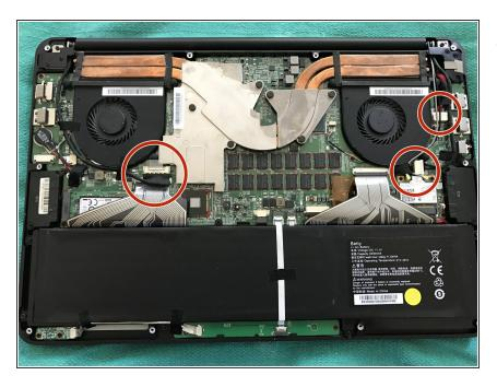
Reconnect cables. (Route these cables in a way that would prevent getting crushed against the bottom cover)
