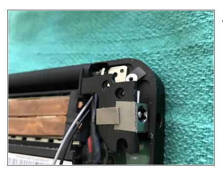
Unscrew right side screws, (you have to lift the charging port out of the case to fully release the hinge)
