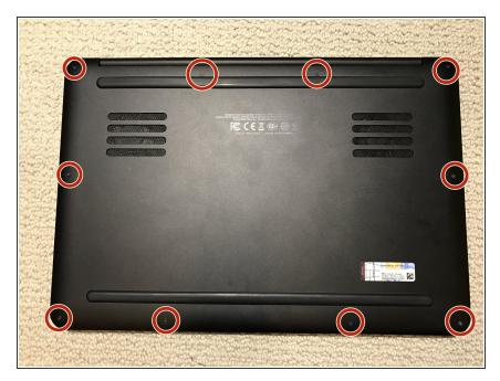
unscrew the 10 (T5) torx screws to release the back panel. Be sure to fully drain your laptops battery or disconnect the battery before tampering with the internal components.
