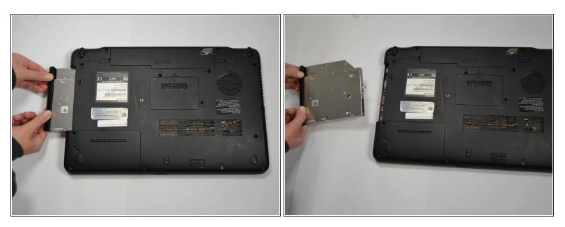
• Remove the optic disk drive from the computer.
