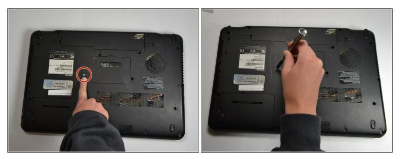
• Remove the 5mm Phillips screw from the bottom of the laptop.
