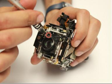
• Unscrew the 5.5 mm JIS #00 screw that is holding the lens to the whole camera.
