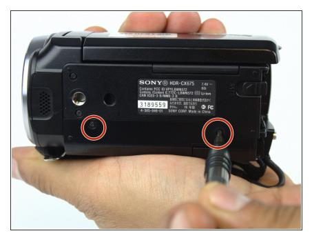
Remove the two 5.5mm JIS #00 screws with the bottom of the camera facing up.
