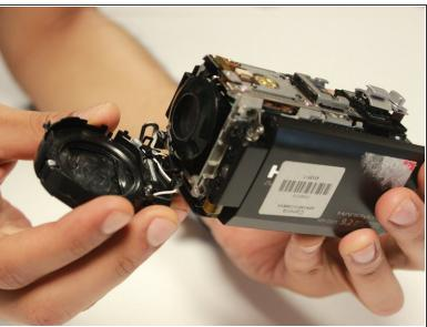
Hold the camera with your left hand, and gently remove the shutter assembly part.
