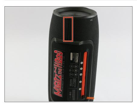
Locate the seams next to the 'feet' on the bottom side of the device.
