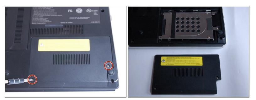
Use a Phillips #00 screwdriver to remove the two 7.7 mm screws from the hard drive cover and place it to the side.
