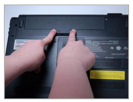
• Slide the two latches towards the center of the battery to release it.
