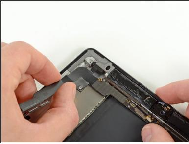
Holding onto the ribbon cable of the headphone jack assembly, carefully pull the assembly parallel to the iPad, toward the bottom of the device.
