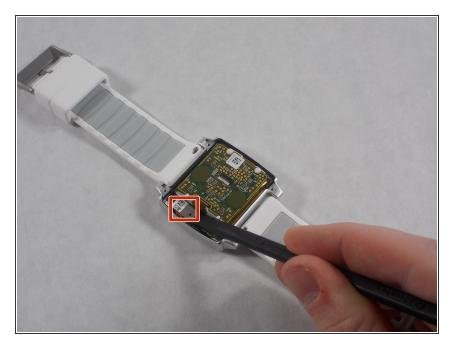
Disconnect the ribbon cable on the left side of the motherboard by using a spudger.
