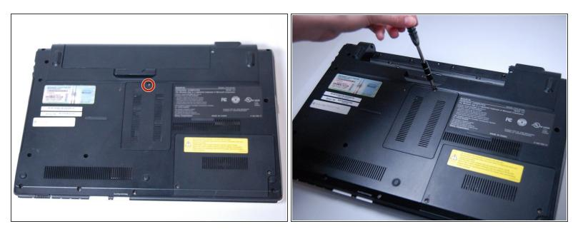
Using a Phillips #0 screwdriver, remove the one screw (Length: 7.7 mm) that is covering the RAM.
