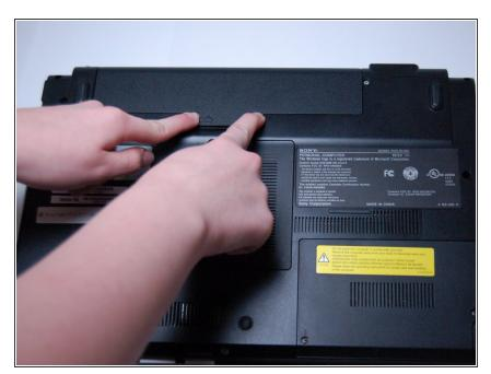
• Slide both latches to the center of the laptop in order to release the battery.
