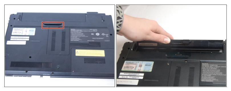
Use your fingernail or a plastic tool to lift the battery. Rotate the battery up and away to remove from the laptop.
