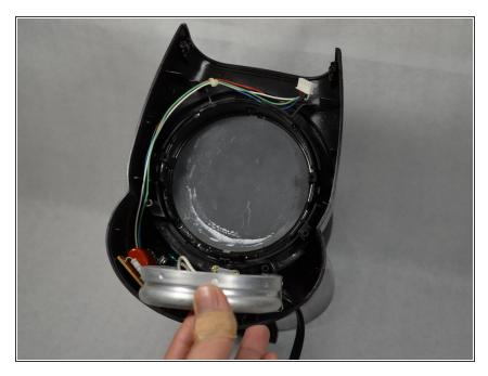
• Pull heating element out of the way.
