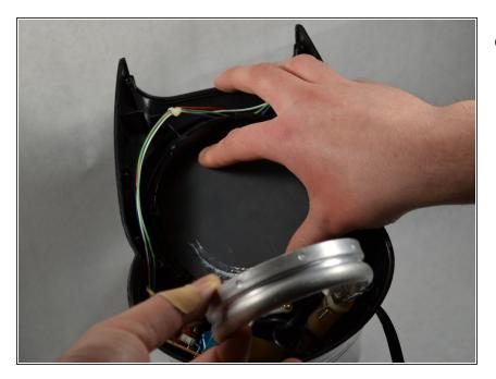
• Twist warming plate clockwise so that the tab is out of place. Remove warming plate.
