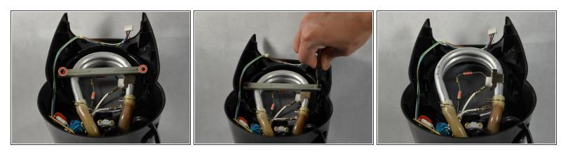
Using a Phillips #1 screwdriver, remove 12mm screws from heating element bracket and remove bracket.
