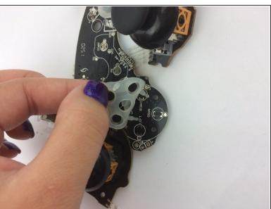
Remove two button padding from the back of motherboard.
