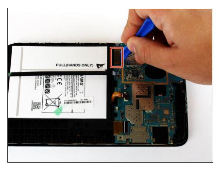
Use the plastic opening tool to pry up the tab holding the motherboard in place.
