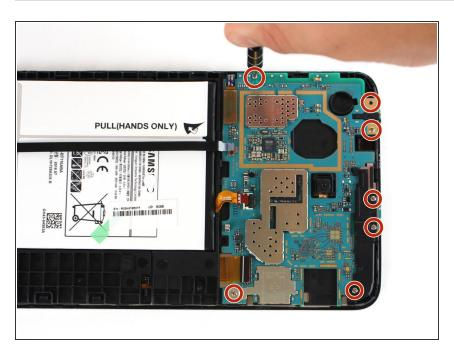
Remove the seven 4mm PH000 screws holding the motherboard in place.
