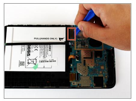
Use the plastic opening tool to pry up the tab holding the motherboard in place.
