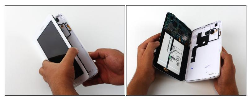
After separating the latches holding the screen and case together, slowly take the screen off the case.
