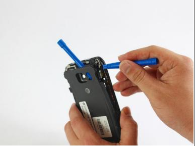
• Insert a plastic tool to pry open the black and beige piece covering the volume button connection.
