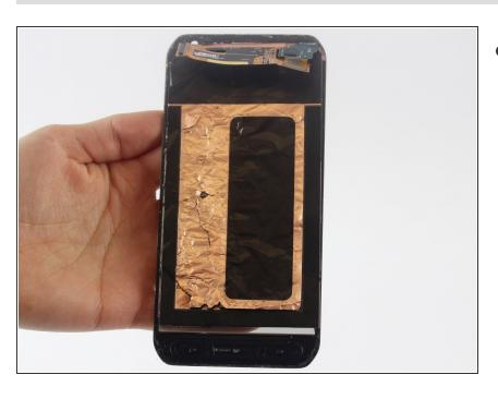
Remove the display assembly (LCD and Digitizer).
