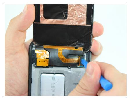
Undo the screen connection with a plastic tool.
