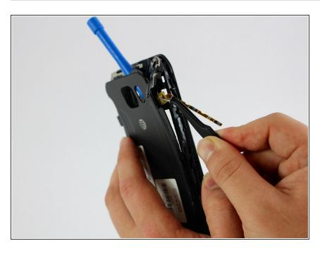
Insert the tweezers under the contact points to undo the connection.
