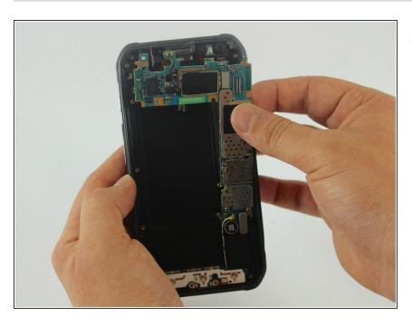
Remove the motherboard from the rear case.
