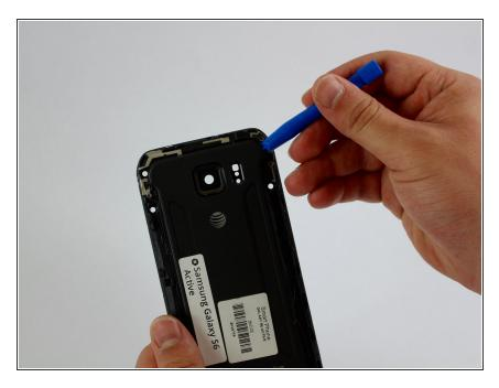
Insert a plastic tool between the frame of the phone and the back cover at the top right corner.
