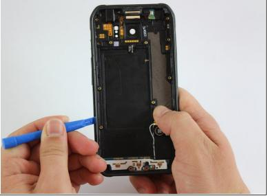
Once you see a large enough gap, insert a plastic tool between the frame and the plastic cover and slide it around the phone to separate both components.
