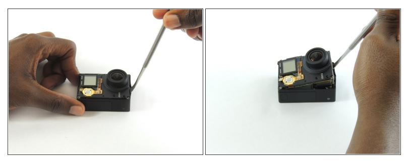
Insert a metal spudger between the back plastic housing and the camera board assembly. Working
