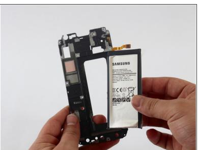
Remove the battery from the frame.
