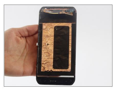
Remove the display assembly (LCD and Digitizer).
