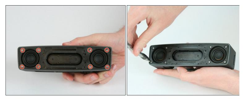
• Remove the eight 9mm T9 Torx screws from the front of the device.
