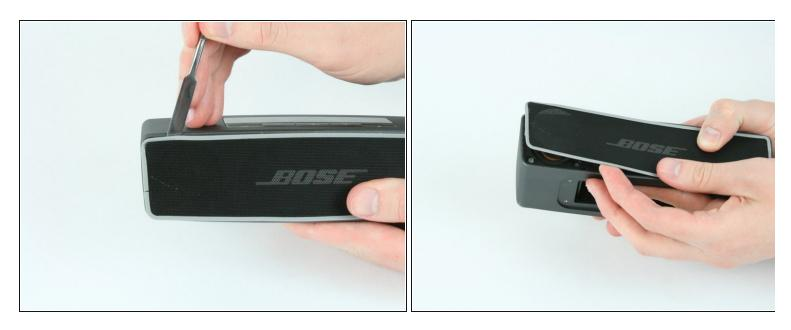
Removing the device front grille with a metal spudger, starting in one corner and working around the border.
