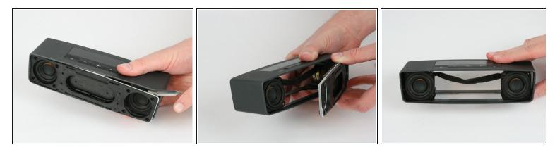
• Use the metal spudger to remove the front case panel.
