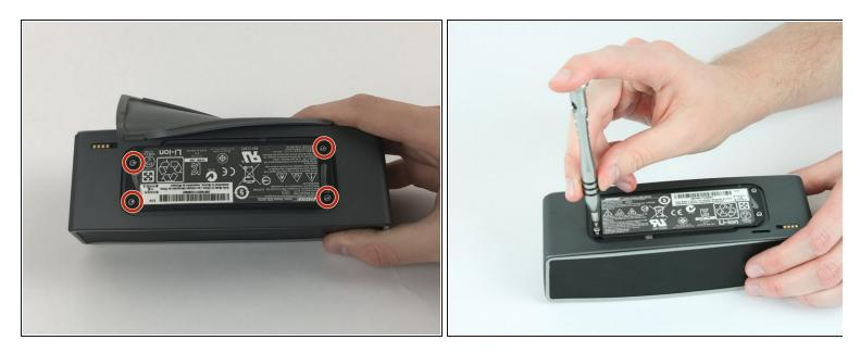
• Remove the four 6mm T9 Torx bit screws from the corners of the battery.
