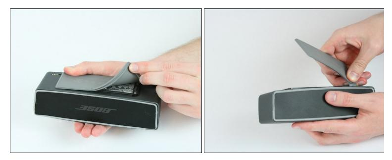
• Gently remove the rubber base from speaker by pulling around the edges.
