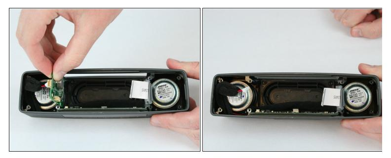
• Remove the power supply board by sliding it outward from the device.
