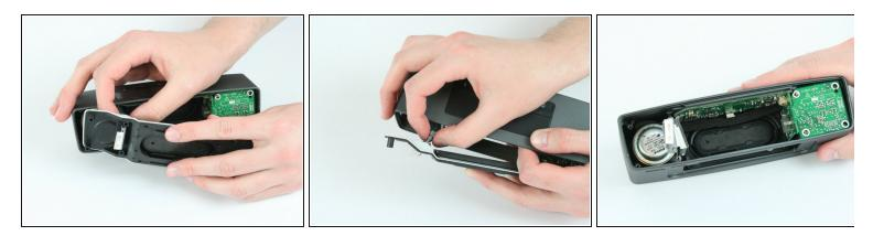
• Pull the ribbon cable through the rear case wall.
