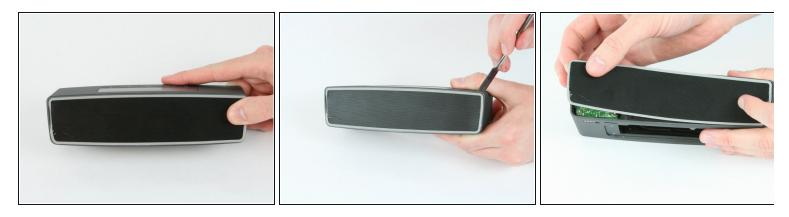
• Remove the rear grille with a metal spudger, starting in one corner and working around the border.
