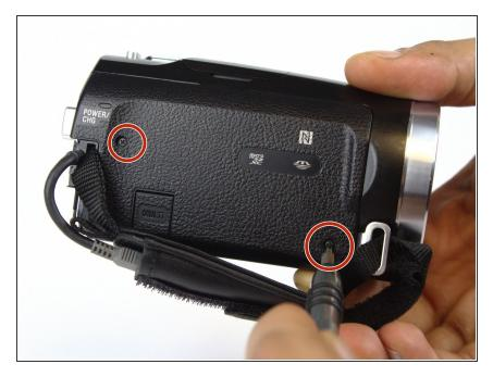
Turn the camera to the handgrip side and unscrew two of the 5.5mm JIS #00 head screws using the JIS #00 head screwdriver.
