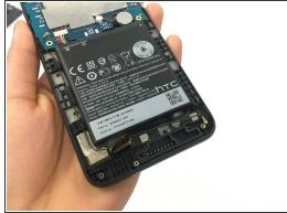
Pry up the circuit board and pull it out using a pair of precision tweezers.
