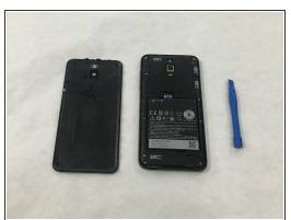
Using a plastic opening tool, take off the back cover of the phone.
