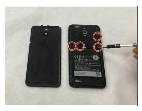
Remove the four black 4mm torx screws using the Torx T5 bit.
