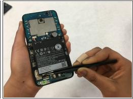
Peel back the gray adhesive strip using the precision tweezers.
