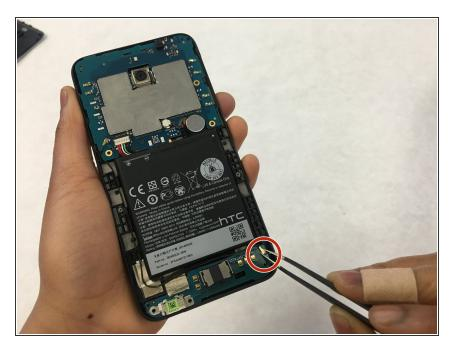
Using a pair of tweezers, disconnect the antenna wire.
