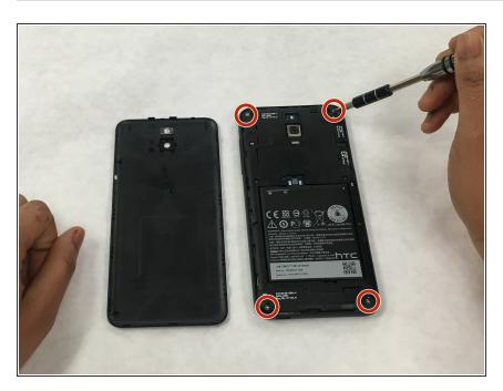
Remove the four silver 5mm torx head screws using the Torx T5 screwdriver.
