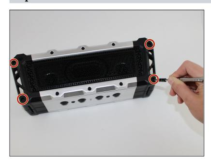
Remove the four 3 mm screws located in each corner using a 3 mm Hex screwdriver.
