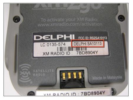
After removing the battery cover and battery, the device information is located near the battery connections highlighted in red.
