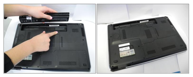
• Carefully pull out the battery while holding the latch to the open position with your finger.
