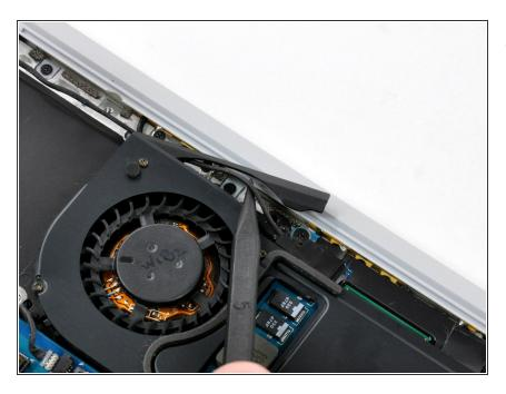
Deroute the microphone cable away from the channel in the fan.
