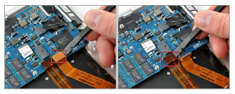
Use a spudger to pry the AirPort/Bluetooth and trackpad control cable connectors up off the logic board.
