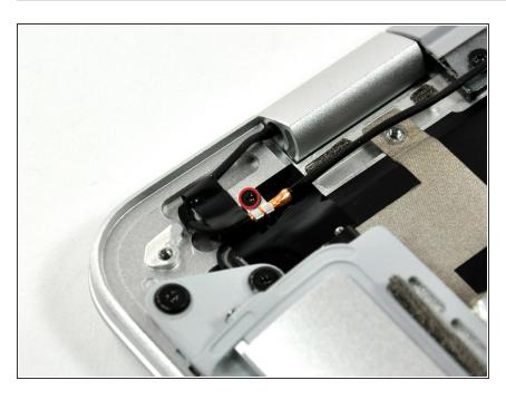
Remove the single Phillips screw securing the microphone cable ground loop to the upper case.
