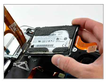
Lift the hard drive assembly out of the upper case.
