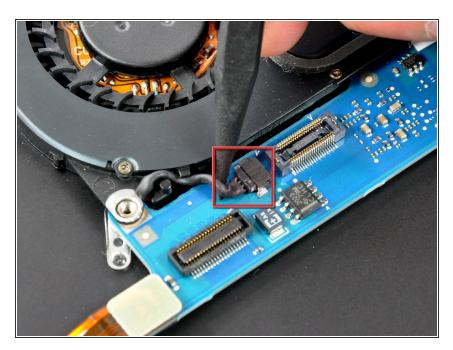
Use the tip of a spudger to pull the fan cable connector straight away from its connector on the logic board.
