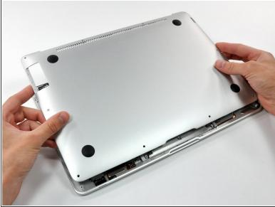
Slightly lift the lower case near the vents and push it toward the rear of the computer to free the mounting tabs.
