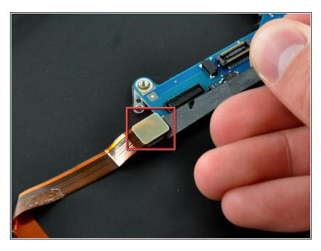
Use a spudger to pry the audio cable connector up off the logic board.
