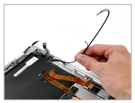
Peel the antenna cables up off the adhesive securing them to the upper case.
