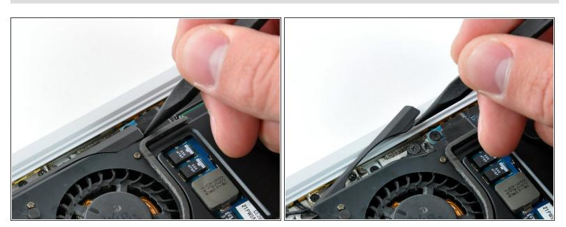
Use the tip of a spudger to move the cosmetic fan cover aside.
