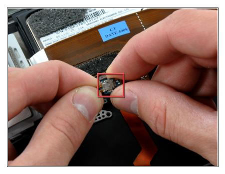
Disconnect the audio out cable from its socket on the port hatch ribbon cable.
