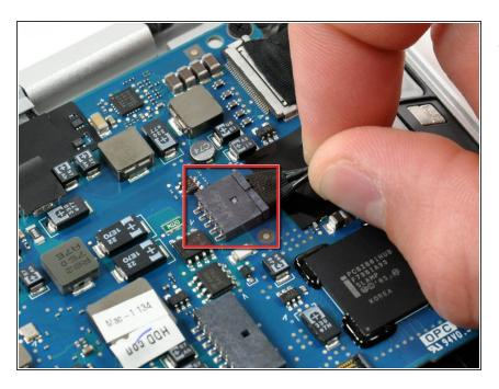
Disconnect the DC-In cable by pulling its connector straight away from the socket on the logic board.
