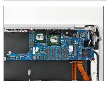
Remove the three Phillips screws securing the logic board to the upper case.
