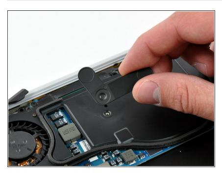
Lift the processor clamp off the heat sink.
