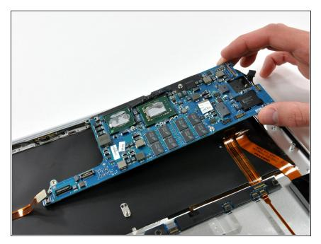
Lift the logic board out of the upper case.
