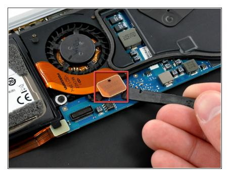
Use a spudger to pry the hard drive cable connector up off the logic board.
