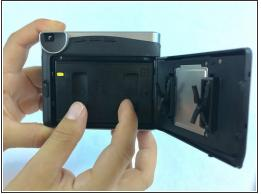
Unlock the back cover. It should automatically spring open. If there is an old film cartridge loaded in the camera, remove it.
