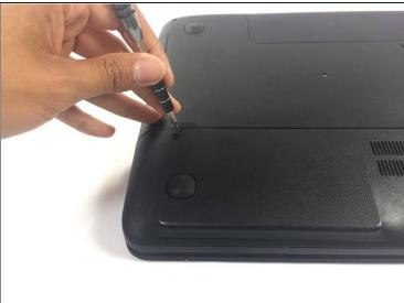
Remove the two screws securing the access panel to the laptop.
