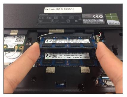
RAM should pop up at about 45 degrees. Pull outwards with fingers on the side of the RAM to remove.
