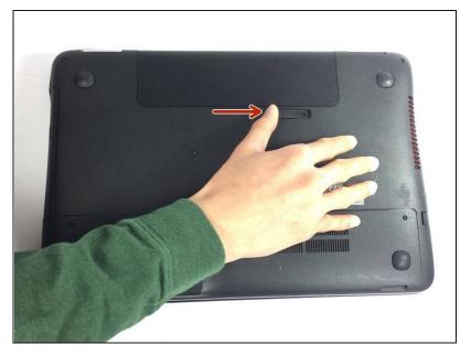
Push the latch found below the battery to the unlock position.
