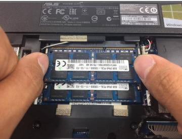
Place thumbs on the locking tabs of both sides of the RAM stick and push outwards to unlock.
