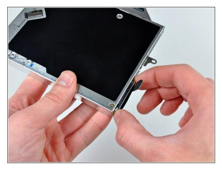
Pull the optical drive cable connector away from the body of the optical drive.
