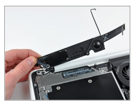
Carefully rotate the rear speaker assembly (with AirPort/Antenna cables still attached) out of the lower case.
