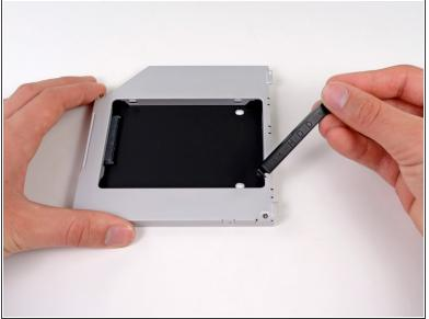
Remove the plastic spacer from the optical bay hard drive enclosure by pressing in on one of the clips on either side and lifting it up and out of the enclosure.
