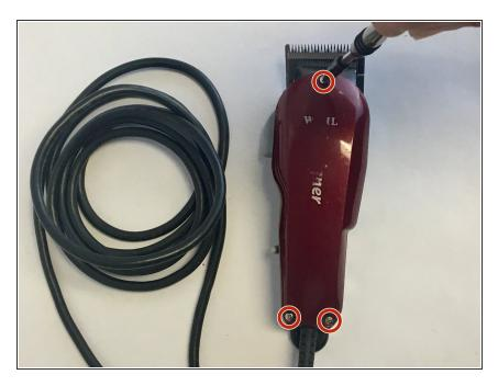
Unscrew the three 12mm black JIS screw found on the red side of the the device with a JIS #1 driver.
