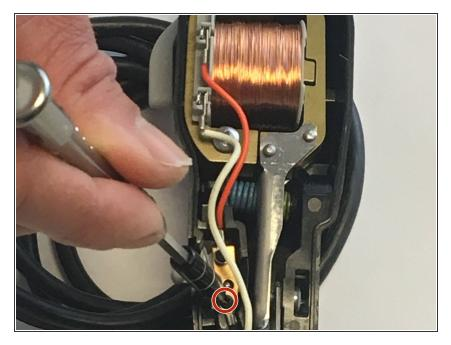
Unscrew the 5.556mm screw with a JIS #0 screwdriver. (Black Screw located at power switch)
