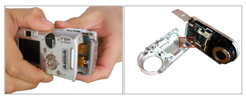
• Carefully separate the front casing from the camera body.
