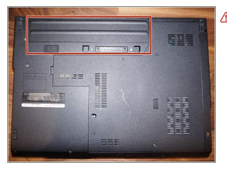
Be sure to remove the battery to prevent any electrical shortage.
