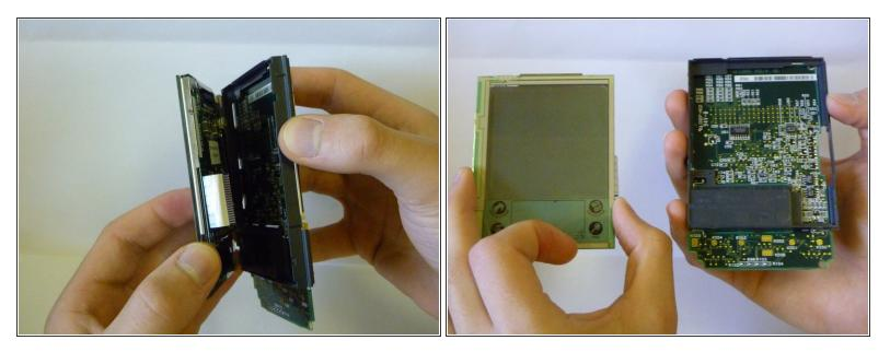
• The screen is now disconnected from the rest of the device and can now be removed.
