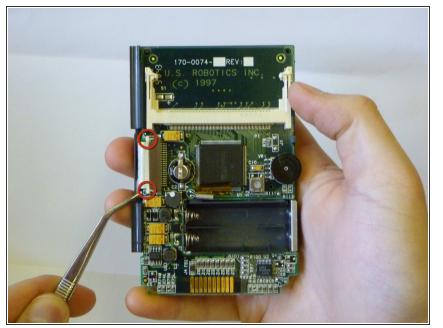
• Looking at the back of the device hold one of the white tabs on the ribbon cable connector down and use tweezers to push in the other white tab toward the device at the same time.
