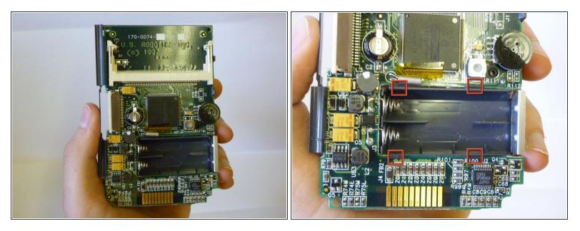
• Depress the tabs around the battery casing so that the battery casing can slide through the rectangular slot on the motherboard - opposite of the metal plate.
