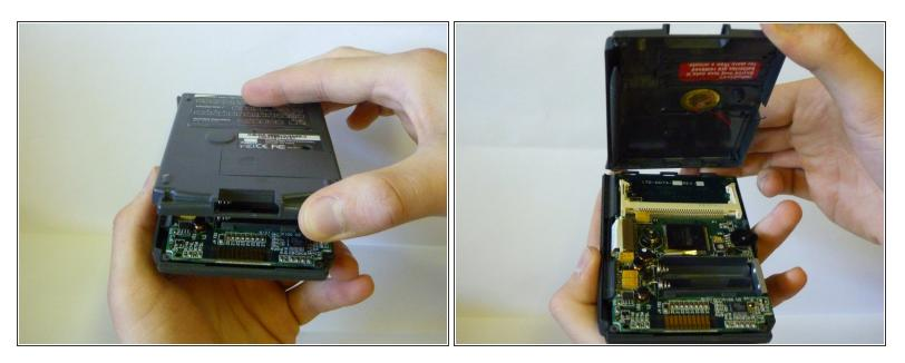
• Pull the back cover from the bottom of the device and separate the interlocking tabs on the top to remove the back cover.
