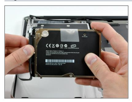
Remove the hard drive from its cable by pulling the cable connector straight away from the drive.
