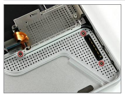
Remove three 2 mm Phillips screws securing the battery connector cover to the upper case.
