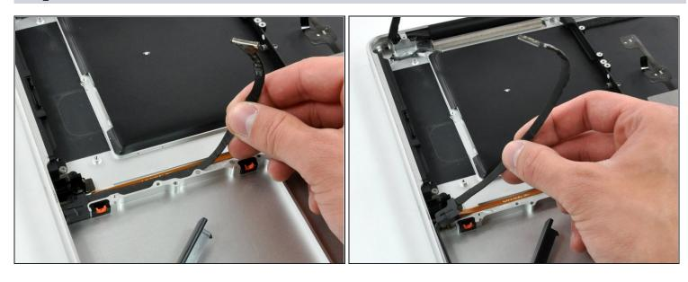
Peel the hard drive cable from the adhesive securing it to the upper case, and maneuver the plastic retaining block out of the upper case.
