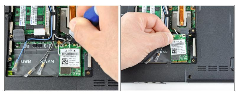
• Remove the 3.70 mm Phillips #1 screw securing the card to the laptop.
