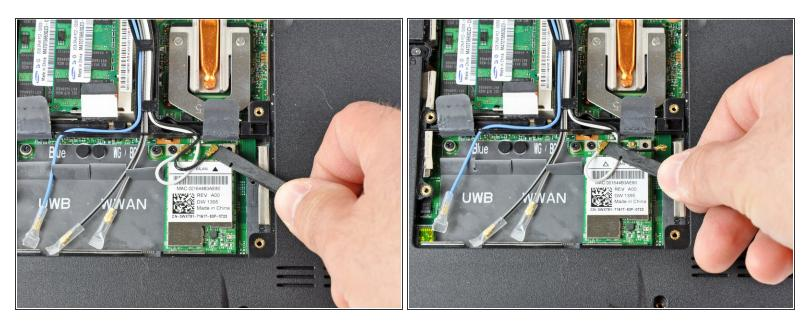
Use the flat end of a spudger to gently pry the black and white antenna connectors off the Wireless Mini-Card.
