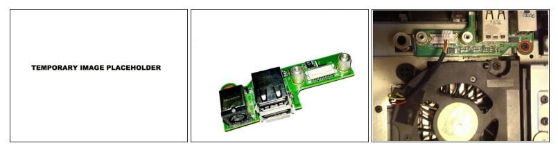
Unscrew the single screw holding the DC charger board into the laptop and lift it out.
