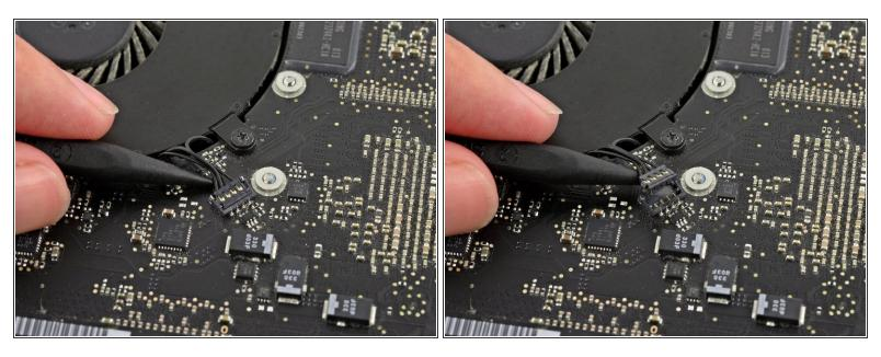
Use a spudger to pry the fan connector straight up and out of its socket on the logic board.
