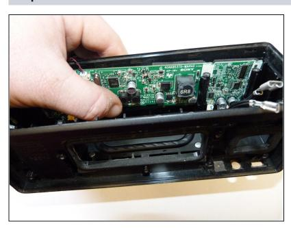
Use your fingers to pull the board upwards while the speakers top is facing downwards. In doing so, use more force than you are comfortable with. (Do NOT worry. The board slides upwards, regardless of the friction that may seem like it is keeping it from sliding out.)
