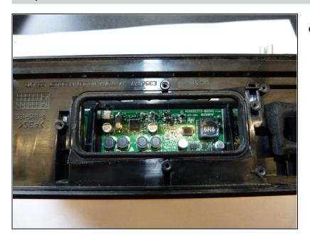
Locate the Motherboard through the hole in which the battery pack normally rests.
