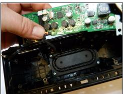
Once the Motherboard has been removed, you are free to remove all of the wires that are connected to it. Gently pull on the clips where the wires insert into the board to remove all of the wires.
