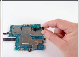
Gently pull the rear camera out of the flex cable socket.
