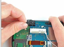
Pry up the right shoulder button casing with a spudger and set it aside.
