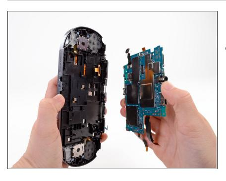
Completely separate the motherboard from the case. Set the case aside.
