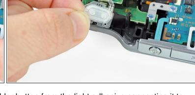
Using a spudger, gently peel up the left shoulder button from the light adhesive connecting it to casing.
