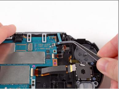
Using tweezers, gently pull the blue power flex cable out of the socket, and rest it out of the way.
