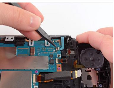
With the help of a spudger, lift and release the tab on the blue flex cable socket.
