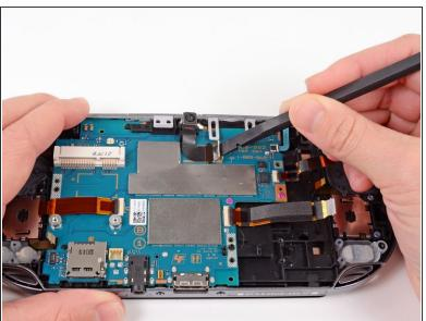
Release the camera flex cable socket by prying up on the tab with a spudger.
