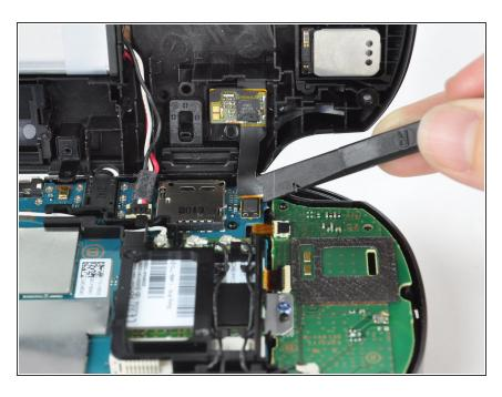
Using a spudger, free the touch screen controller flex cable by gently prying up the connection.
