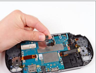
Carefully lift and remove the camera, sliding the flex cable out of the open connector socket.
