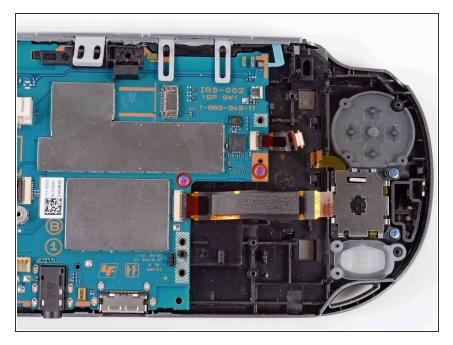
Using a Phillips #00 screwdriver, remove the two pink, 4.4mm screws securing the motherboard.
