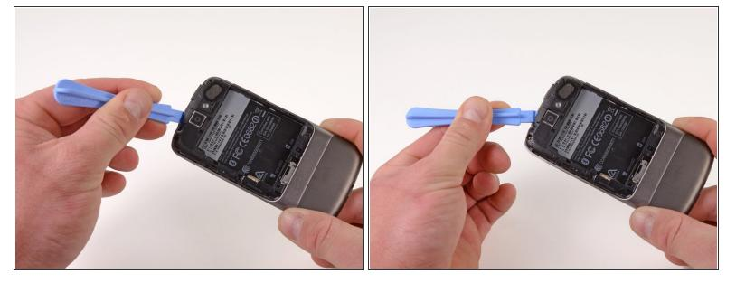
Pry the top tab of the battery housing.
