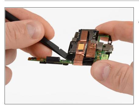
Use the spudger to lift the SIM card tray connector off the motherboard.
