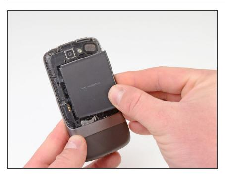
Pull the battery up and out.
