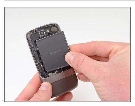
Pull the battery up and out.
