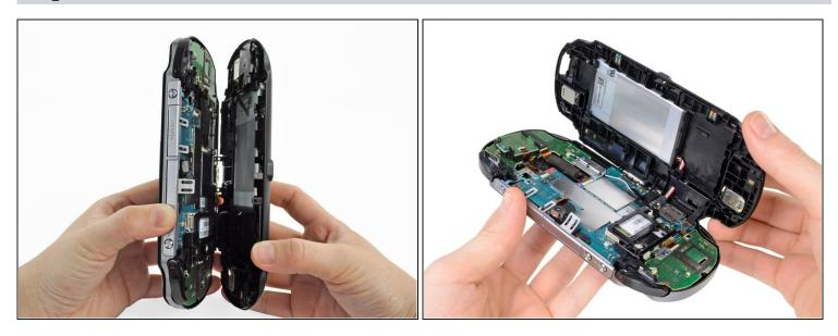
• Gently separate the two cases, minding the battery and the touch screen controller connectors holding the two cases together.
