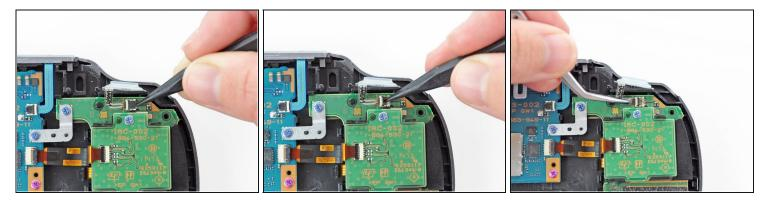
• Release the left shoulder button flex cable socket by using a spudger to pry open the tab.
