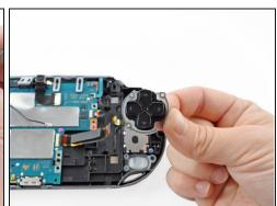
• Using <u>tweezers</u>, peel up and remove the directional pad.
