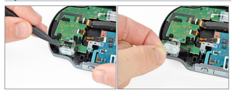
• Using a spudger, gently peel up the left shoulder button from the light adhesive connecting it to casing.
