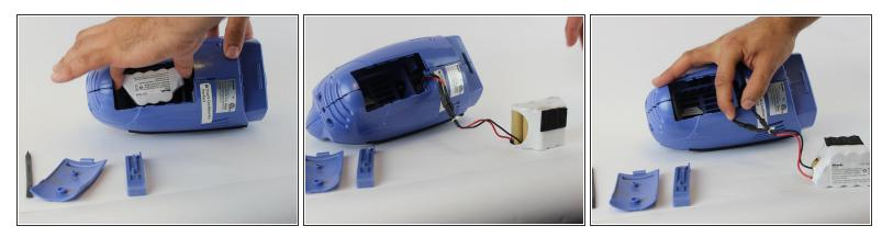
• Pull out the battery and then disconnect the battery at the quick disconnects.
