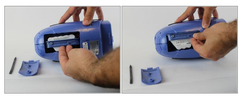
• Once the battery cover is removed slide the battery mount upwards and pull it out.
