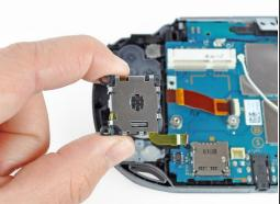
Using a spudger, gently pry the joystick out of the back casing assembly.
