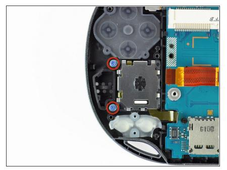
Using a Phillips #00 screwdriver, remove the two 5.0mm, blue screws from the right joystick.
