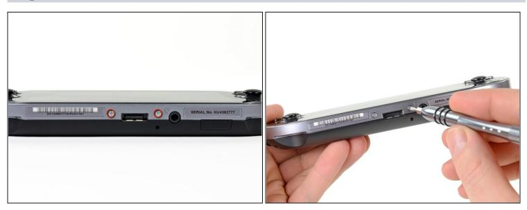
• Remove the two 5.4mm Phillips #00 screws on the bottom of the device near the charging port.
