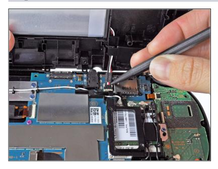
• Free the battery cable by gently prying up on the connection with a spudger.
