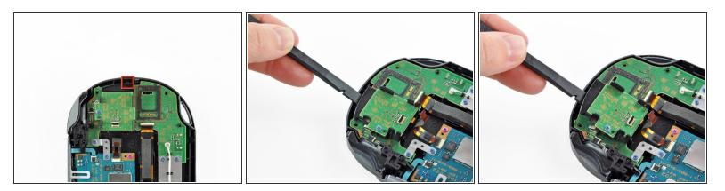
Use a spudger to release the plastic tab along the inside of the case and gently pry up the SIM card reader.
