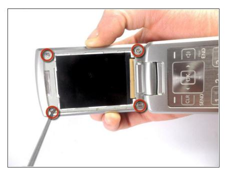
Unscrew the four corner 3.21mm screws to separate the the top cover of the phone
