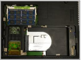
Using a plastic opening tool, pop off the L shaped panel.
