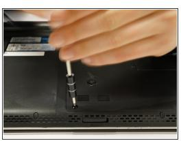
Using a size 0 Phillips screwdriver, remove two (2) 5mm screws from the L shaped back panel.
