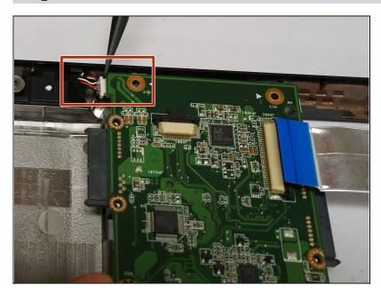
Disconnect one (1) red/black connector wires by prying them out with the nylon spudger.
