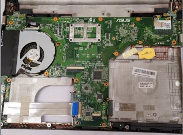
• Remove the keyboard from the computer to reveal the motherboard.
