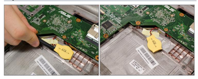
• Disconnect one (1) white/red/black connector wire by prying it up with the spudger.
