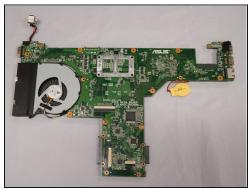
• Insert index fingers underneath the motherboard in the top corners of the motherboard. Slowly move your fingers toward the center of the board while lifting up gently. The motherboard will lift easily from the device casing.
