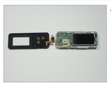
You can now safely remove the front case cover from the device.
